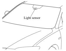
> The light sensor also works as a rain sensor for the auto-wiper control. Keep hands and scrapers clear of the windshield when the ignition switch is in the ON position as fingers could be pinched or the wipers and wiper blades damaged when the wipers activate automatically. If you are going to clean the windshield, be sure the wipers are turned off completely - this is particularly important when clearing ice and snow - when it is particularly tempting to leave the engine running.
